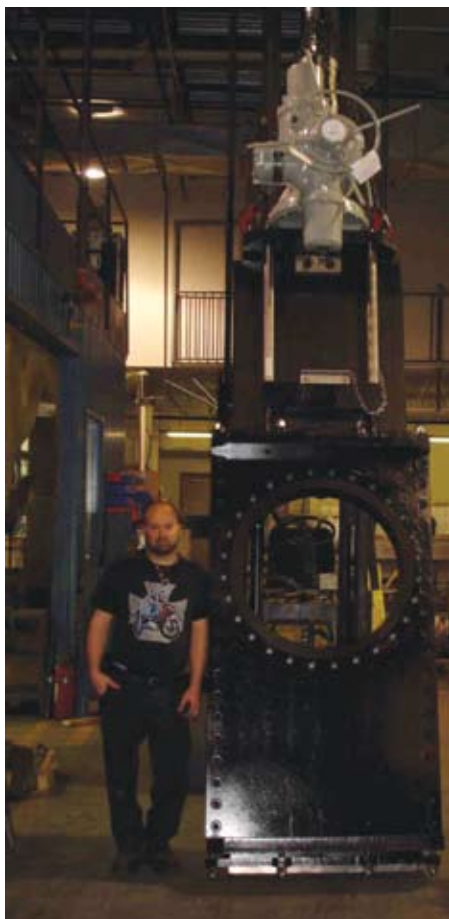
30" ANSI 150LB O-Port Valve fully rated to 285psi working pressure. Used on scale forming vapor lines.
