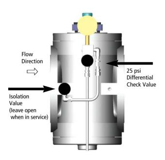
The above system is designed to relieve any excess rise in pressure, within the body cavity, due to terminal expansion of the liquid within the cavity, when the valve is in the closed position. The relief valve is set to open at 25PSI or above and bleeds excess pressure to the upstream side.
