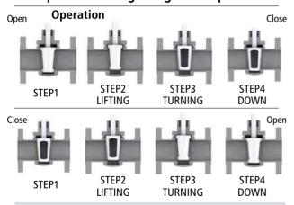
The body and plug contacts directly metal-to-metal. To prevent the surfaces from galling or abrading the valve is designed to operate as following steps;
